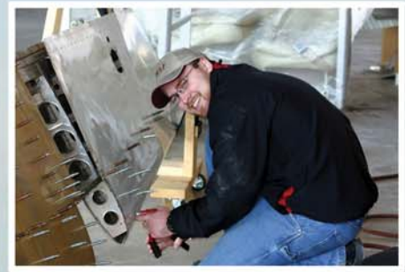
Riveting the horizontal stabilizer back together after removing corrosion inside.
